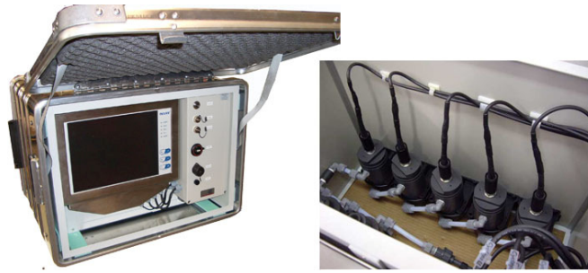
Figure 3: Photo of the pocketFerryBox (left) and of the flow-units (right).
