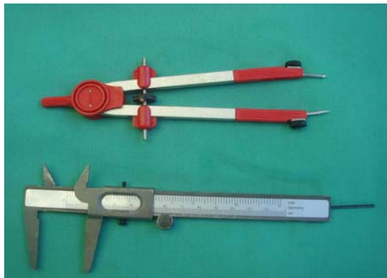
Fig. 2.2: Measurement tools: vernier caliper and circle
