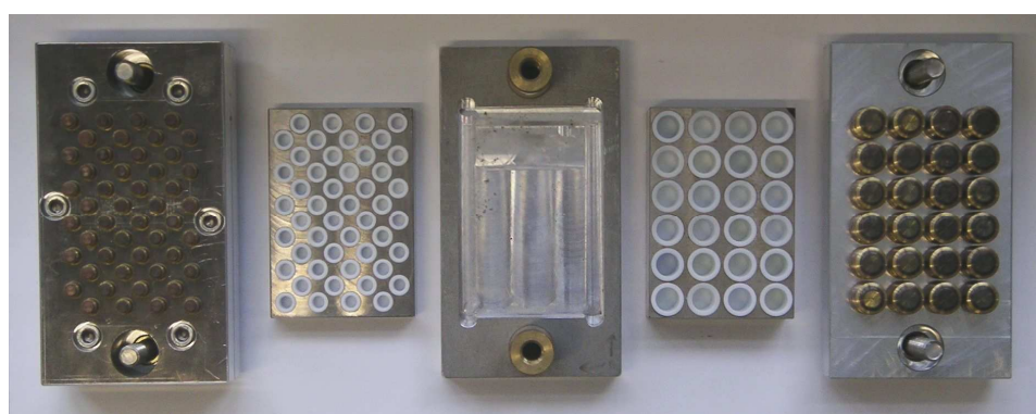
Figure 3.1 Stainless steel HT-multiclaves with 48- and 24-Teflon ® -lined reaction chambers (120 mm x 80 mm) employed by the group of Stock.
