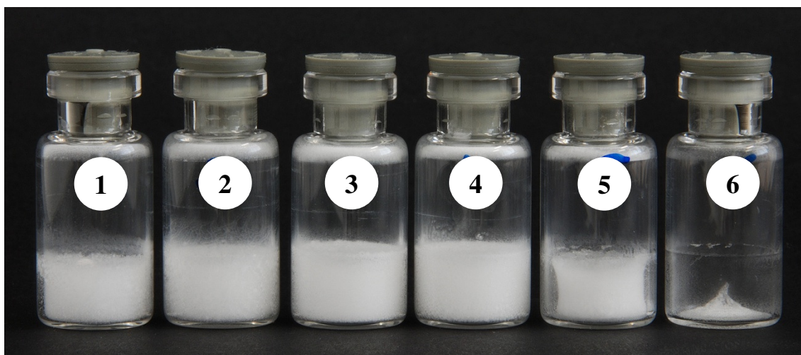
Figure 5.19: Photograph of different lyophilisates containing 100 µg ZOL and 5 mg (1), 10 mg (2), 15 mg (3), 20 mg (4) mannitol, 15 mg trehalose (5) or 15 mg sucrose (6).
