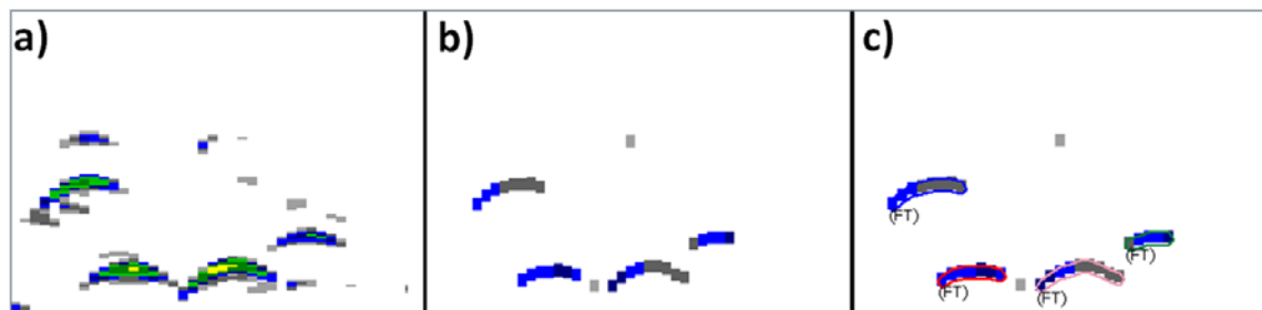
Figure 7: Identification of individual cod from hydroacoustic data from the Bornholm Basin. a) Hydroacoustic raw data as visible on echosounder screen at a threshold of -50 dB. Five typically shaped echotraces consisting of multiple echoes indicate presence of fish. Colors indicate different target strength of echoes. b) After application of a single target identification algorithm with a threshold of -37 dB, only the echoes that are attributed to a single backscattering target with predefined properties remain. Note that one individual fish can scatter multiple single echoes with different target strength. c) The application of a fish-tracking algorithm combines single targets with systematic movement and distribution patterns to a single object (Fish Track, FT) – in this case four individual cod ( Gadus morhua ).
