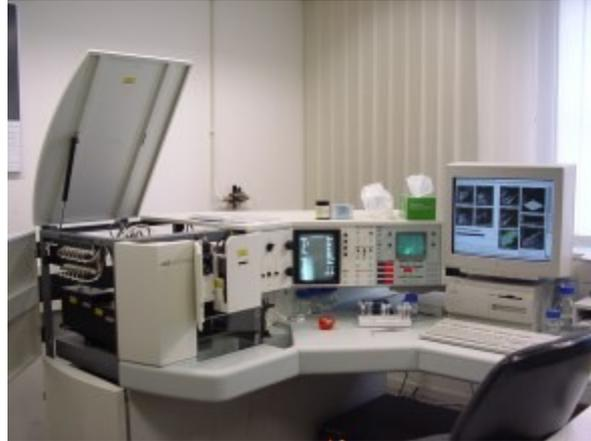
**Figure 2.1.:** Becton Dickinson FacsVantage (Flowcytometer) in **Research and Technology Centre (FTZ), Working Group Applied Physics/ Marine Technology (APM)**. The specification of the system: Argon ion plasma laser (488 nm) and an HeNe-Laser (633 nm) for the excitation, 3 scatter and 4 fluorescence detectors on the emission side, sort head implemented.
