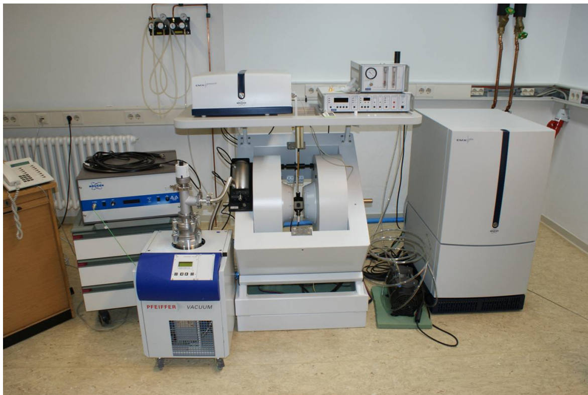
Figure 5.3.: Picture of the cw X-Band EPR spectrometer at the Institute of Inorganic Chemistry, Kiel University.
