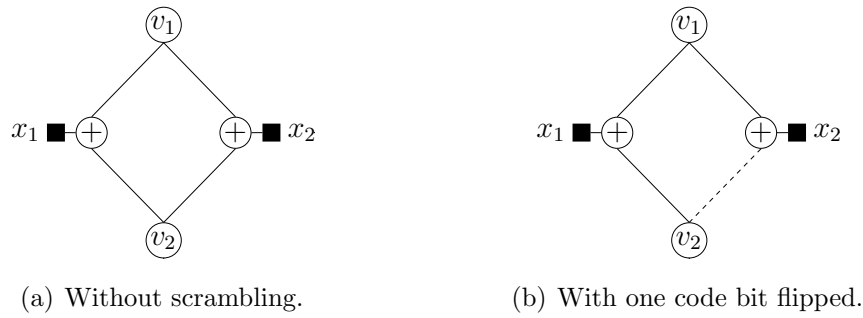
Figure 6.18: Factor graph for repetition-coded SM-EPA, SF = 2 , N = 2 , K = 2 .
