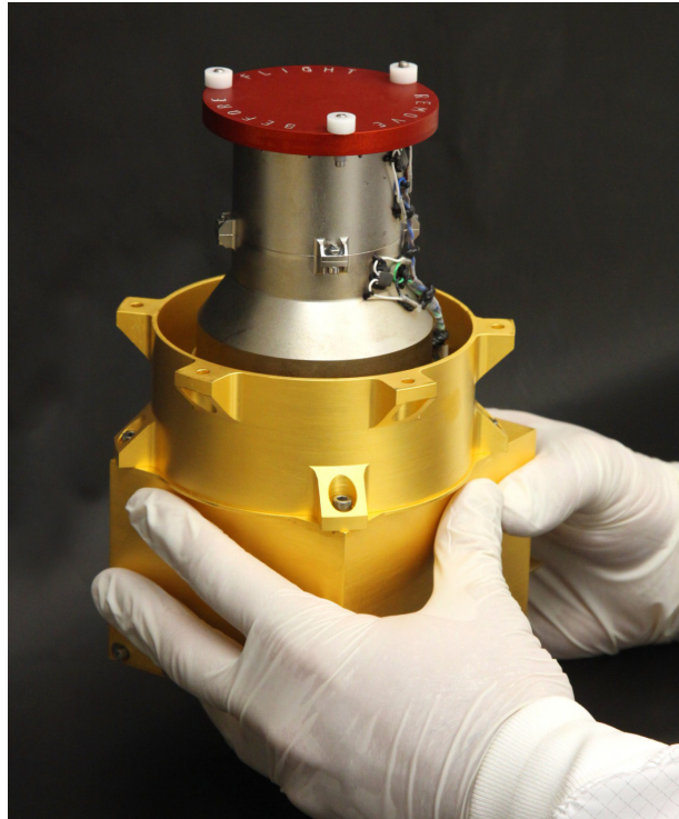
Figure 1.2: The RAD instrument before being integrated into the MSL rover. The red protective cover on top of the instrument was removed before flight. Provided by NASA photojournal .
