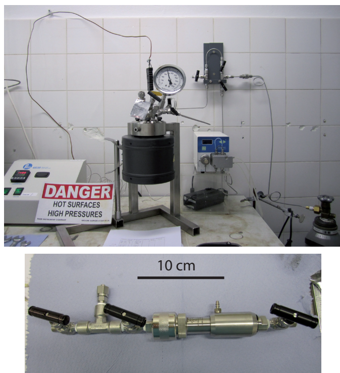
Figure A.3: Experimental setup of the used PARR reactor with heating control (top left), reactor with furnace and pressure control (top middle), Knauer pump system and gas bottle (top right) as well as the sampling system (bottom)
