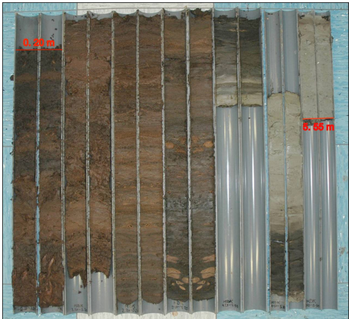
Figure 2. Sediment sequence of the core MDK 0.20–5.55m (kettle hole mire 'Brunsrade Moor'). Two parts of the core in length and both half are shown
