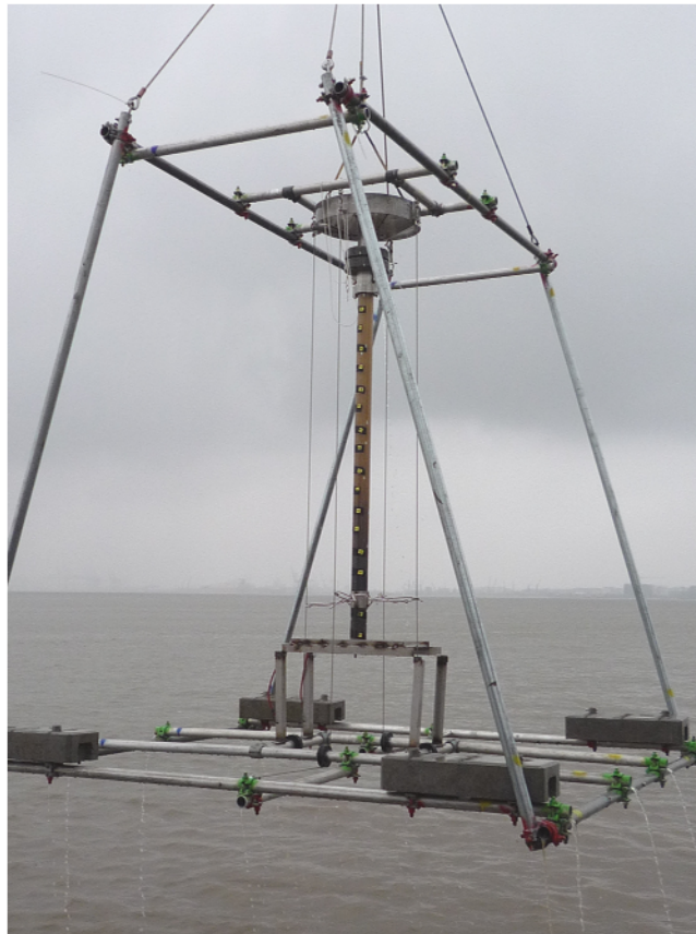
Figure 4.2: Rumohr-type gravity corer (2 m length) with a special constructed weighted steel frame (~3 x 3 x 3 m) and a closure system for sampling at current velocities up to 1.5 m/s.
