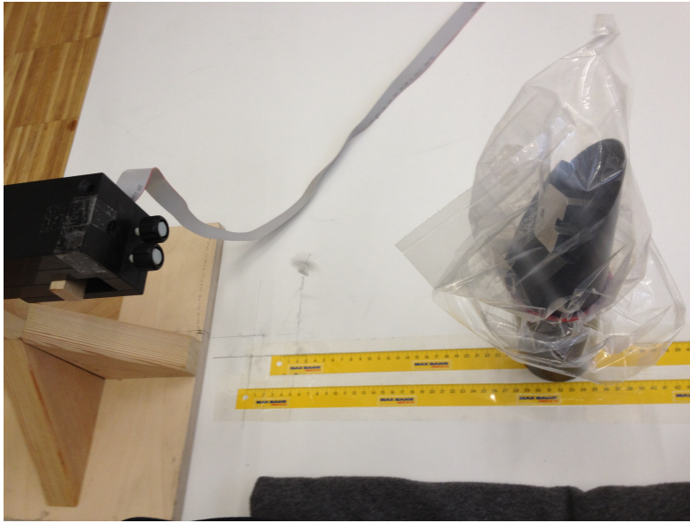
Figure 6.24.: Placement of the pedestal EPT1 →MAG IBS. The pedestal holds a dummy of a magnet system and is covered with a plastic bag. On the wooden plate one can see the drawings of the perpendicular point of the barycenter of the three sensors and the yellow measurement tape.
