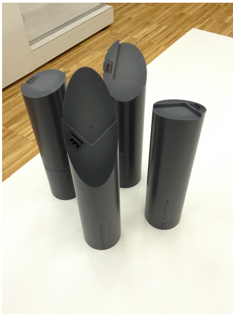
Figure 6.22.: Four plastic pedestals to hold the magnet systems.
