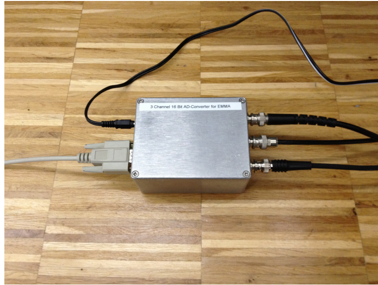
Figure 6.13.: The box, that contains the AD-converter for EMMA. On the left the box is connected to the iOS device and to the power adapter (black), and on the right to the three outputs of the magnetometer.
