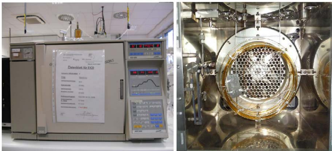
Figure 2.2: FISIONS 8000 gas chromatograph with ECD detector was used for discrete samples analysis. GC-column (right side) parameters: 60m, 0.25mm, RTX-VGC.
