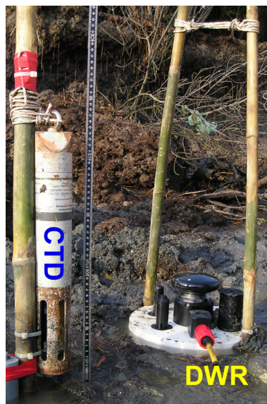
Figure 5.3. In-situ deployment of a CTD (Conductivity Temperature Depth) and a DWR (Directional Wave and current Recorder) (delete Midas).
