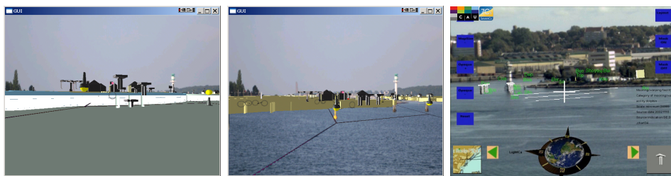
Figure 4.35: Visualizations of the new augmented scene in different types. Left: The fully rendered scene is overlaid onto a video image. The water surface or other objects are not detectable anymore. Furthermore, the objects occlude themselves. Center: An adapted augmentation image is shown. The main orientation aspects like sky, background and ground are visible and furthermore, the interesting data is overlaid and conspicuous. Right: The user's view is shown. The augmentation scene is enhanced with blue buttons to interact with the scene and navigation information in the bottom like a compass, the original 2D sea chart or objects which follow when the user moves in the right or left direction.
