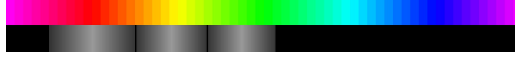
Figure 4.61: Hue spectrum (colored) with probability distributions shown as grey-colored stripes. Dark values belong to low probabilities and bright ones to high values.
