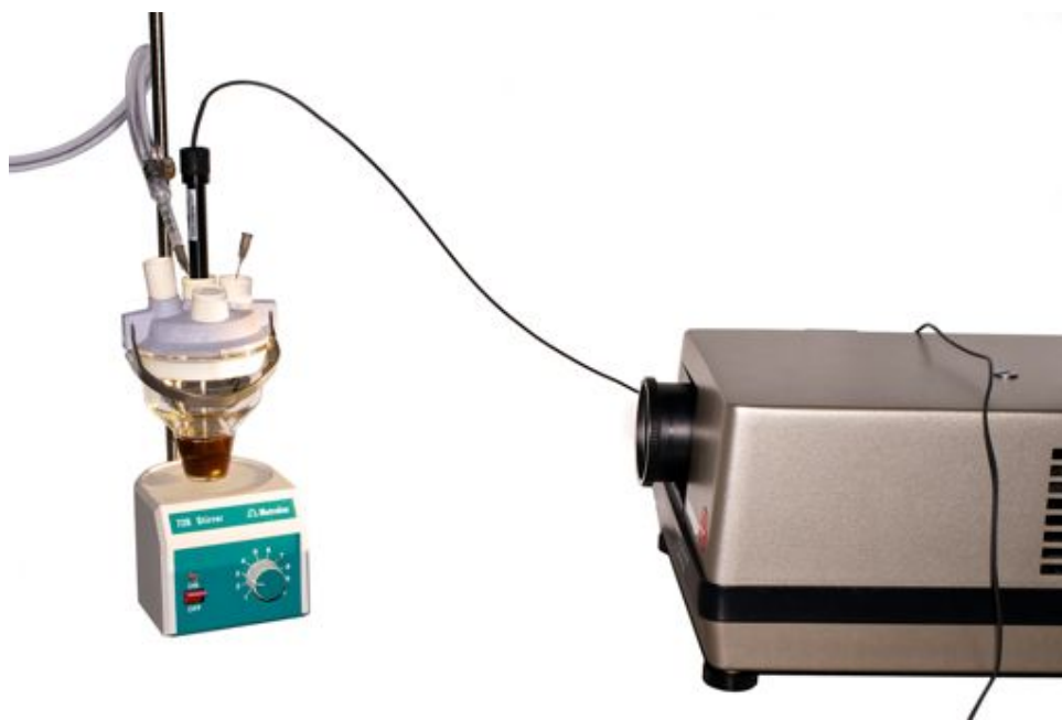
Figure 9.3. Reaction vessel ( left ) and slide projector as light source ( right ) for experiments on water-oxidation catalysis using photochemically generated (\text{Ru}^{\text{III}}(\text{bpy})_3)^{3+} .
