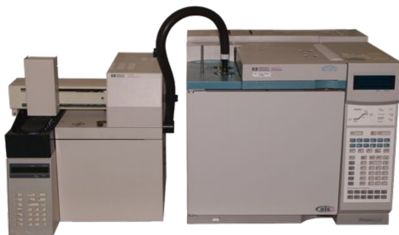
Figure 9.2. Headspace sampler ( left ) for the automatic injection of gas samples from the headspace of the septum vials into the GC ( right ).
