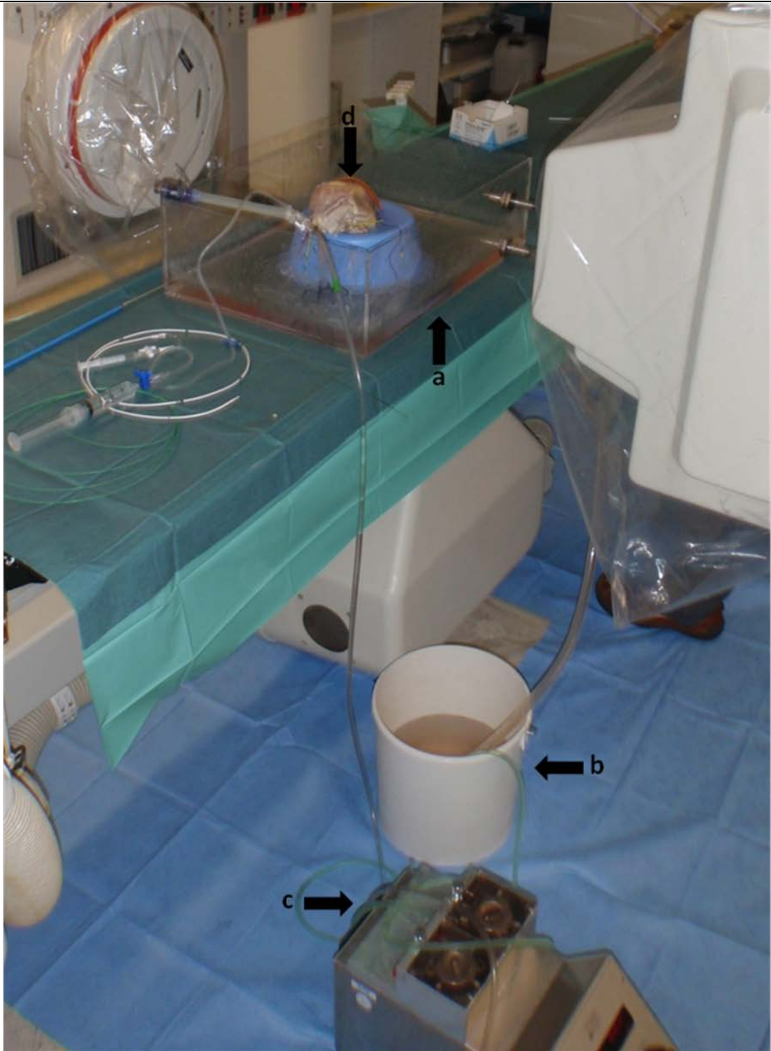
Fig 2.18 The in vitro circulation system. a: Acryl glass box; b: Water recycle pool; c: Rotary pump; d: Porcine heart and its fixation system.
