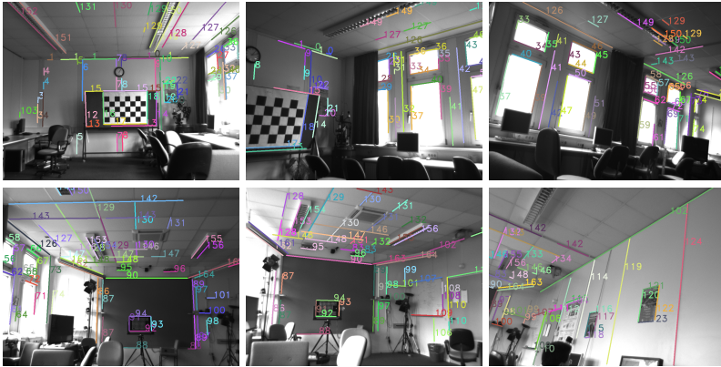
Figure 5.9. Six images taken from the sequence of the laboratory which includes 70 views and 165 lines. Those lines are shown in the images whenever they are detected.
