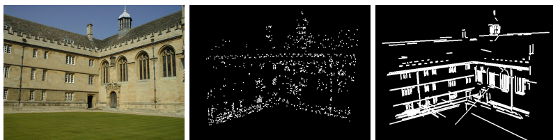
Figure 1.2. An example of the point and line maps. The first picture is a sample image from the Wadham College Dataset ( http://www.robots.ox.ac.uk/~vgg/data/data-mview.html , accessed on 12th, October, 2012). The second picture shows the reconstructed point cloud of the 3D scene and the third picture shows the reconstructed line structure of the 3D scene.
