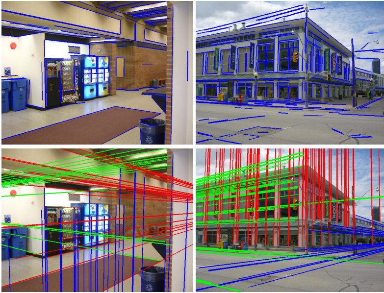
Figure 1.3. Two example images of an indoor and outdoor Manhattan scene. The images are from the York Urban Dataset ( http://www.elderlab.yorku.ca/YorkUrbanDB/ , accessed on 8th, May, 2012). The first row shows the images with extracted lines imposed. The second row shows three orthogonal dominant directions. Lines corresponding to the same Manhattan direction are shown in the same color.
