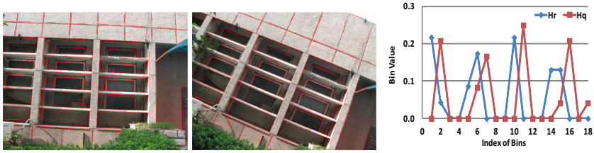
Figure 3.3. Illustration of line direction histograms. The first two images show the reference and query images with detected lines and the plot shows their direction histograms. The resolution of each bin is 20 degrees, so there are 18 bins for each histogram.
