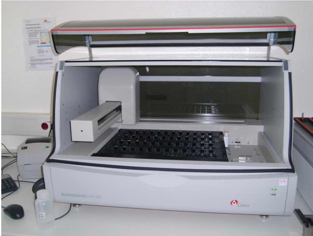
Figure 3: Autostainer Link 48, DAKO, Fermont, Denmark: Automated immunostaining devices can improve standardization and reproducibility of immunohistochemical procedures.
