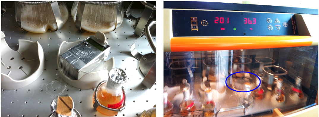
Figure 3.15.: Vibration test with MDT-01-001 in a shaking incubator. The left panel shows the MDT taped to the carrier, the right panel shows the shaker in action and therefore appears to be blurry. The MDT is indicated by the blue ellipse.
