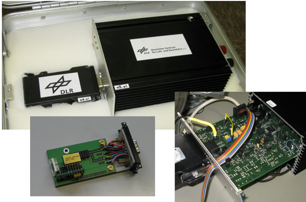
Figure A.2.: Setup of board version 05.01 with preamplifier board 06.01 for measurements during flights (compare Section G.1).
