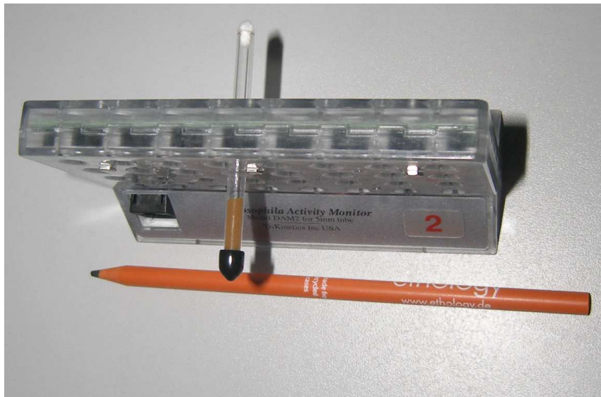
Figure 8: Drosophila activity monitor. It takes 32 individual activity tubes. A single activity tube is shown in place.
