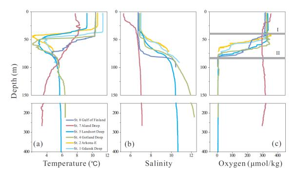
**Figure 5.2** Temperature (a), salinity (b), and oxygen concentration (c) of the studied depth profiles. (I): boundary between the mixed layer and the subsurface halocline layer (~40 m water depth); (II) boundary between the subsurface halocline layer and the anoxic layer (~80 m water depth).
