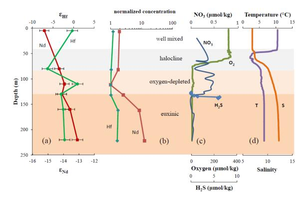
**Figure 5.7** Vertical profiles of (a)  $\varepsilon_{Hf}$  and  $\varepsilon_{Nd}$ , (b) Hf and Nd concentrations (normalized to concentration at 110 m water depth in order to visualize the variability within the oxygen-depleted layer), (c) nitrate, and oxygen concentrations of our cruise, together with H<sub>2</sub>S concentrations obtained in 2010 from a profile close to our station (Dalsgaard et al., 2013), (d) temperature and salinity at the Gotland Deep station.
