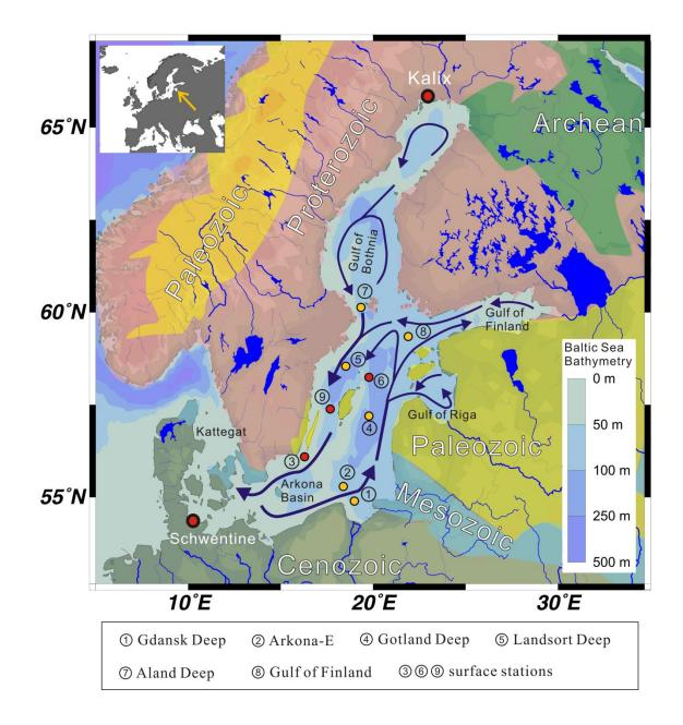
**Figure 5.1** Map illustrating the sampling locations of the GEOTRACES cruise on R/V Oceania in the central Baltic Sea in November 2011, as well as the river water sampling locations (generated using Ocean Data View, Schlitzer, 2012). Red dots represent surface water stations whereas yellow dots represent depth profile stations. Also shown is the simplified geology of the continental area surrounding the Baltic Sea (after Kuhlmann et al., 2004).
