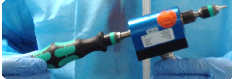
Figure 13: Insertion torque measurement system used for HA performance pilot and main studies.
