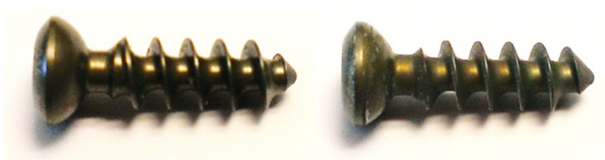
Figure 10 Titanium cancellous bone screw (reference) left and HA coated cancellous bone screw (test) right.
