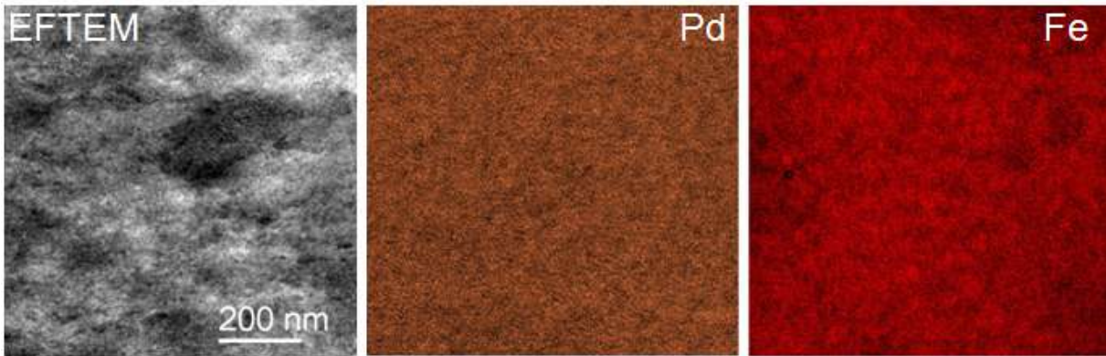
Figure 36: EFTEM micrograph of the sample heated to 550°C. Fe and Pd maps show a homogenous distribution of Fe and Pd.
