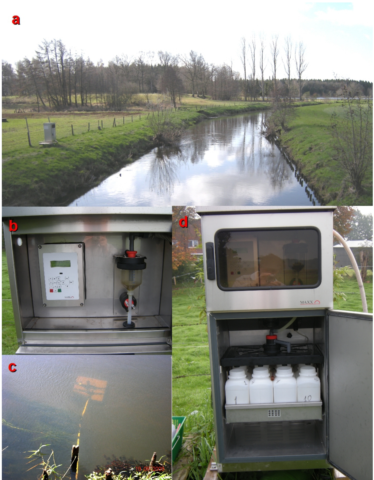
Fig. 4.3 Automatic water sampler MAXX SP III© installed at the gauge Willenscharen (a), central computer and pump collector system (b), water tube collector installed into the river (c), view of the bottles into the automatic water sampler (d).
