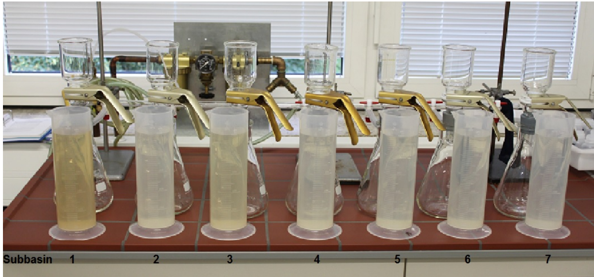
Fig. 5.17 Color yellow "black tea", indicating P link with iron in subbasin 1 and 3.
