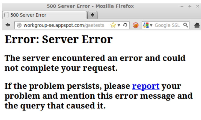
Figure 7.4. Google App Engine displays an error message when running an application that calls the method java.io.File.createTempFile()
