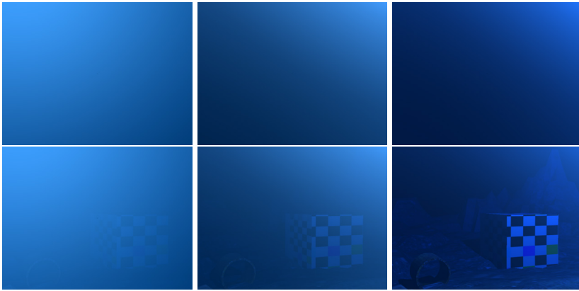
Figure 3.16. The lamp was moved from being directly at the camera to 2 m at the upper right. As Jaffe already concluded in his work, the backscatter portion is causing the contrast to decrease if the lamp is close to the camera. The top row shows the backscatter component and the bottom row the resulting images.
