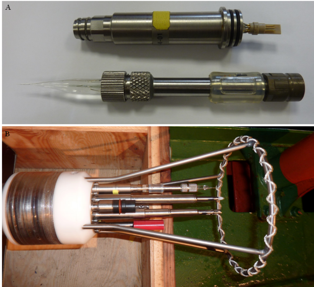
Fig. IV.1. The fast O 2 microsensor system. (A) The main system components: the amplifier housing (top), the in-situ connector system with pressure compensation and the O 2 Clark type microsensor (bottom). (B) Close-up of the MSS system microstructure profiler with mounted the fast O 2 microsensor system and other sensors (described below) prior to deployment.
