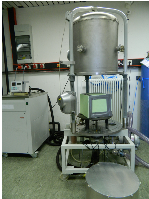
Figure 6.2: The thermal vacuum chamber with the cooling plate and the insulated instrument. The shroud is lying in front of the chamber
