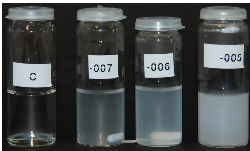
Figure 5.13 0.1% (-007), 0.2% (-006) and 0.8% (-005) DCA solutions added to a 1% Chitopharm S solution (dissolved in 1% acetic acid). Control (C) is the 1% chitosan solution.
