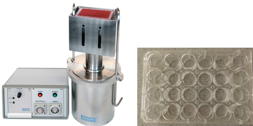
Figure S2. Left: Hielscher UIP250MTP ultrasonic processor; right: view of the modified Greiner Bio-One 24 well cell culture plate with holes of 3 mm diameter drilled through the plates.
