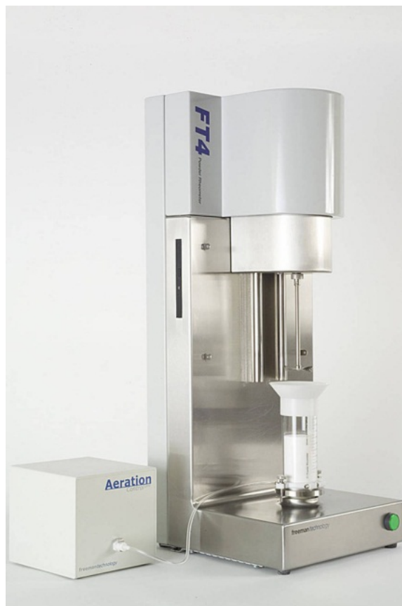
Figure 4.7: Freeman FT4 Powder Rheometer® with Aeration Control Unit
