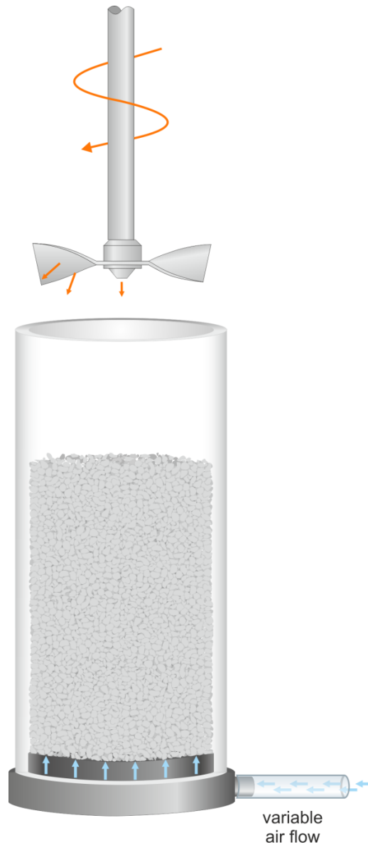
Figure 4.13: Schematic set-up of aeration tests
