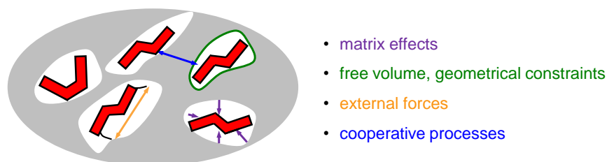
Figure 1.6: Schematic representation of possible effects which act on molecular photoswitches in a complex environment (violet: matrix effects, green: geometrical constraints, orange: external forces, blue: cooperative effects).
