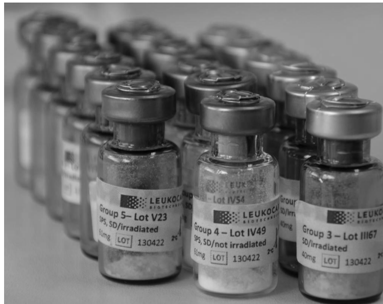
Figure 4.23: Formulations for in-vivo study (Right vial: Group 3 (Pandemrix SD M 25 kGy), Centre vial: Group 4 (Pandemrix SD SPS T final), Left vial: Group 5 (Pandemrix SD SPS T final 25 kGy))
