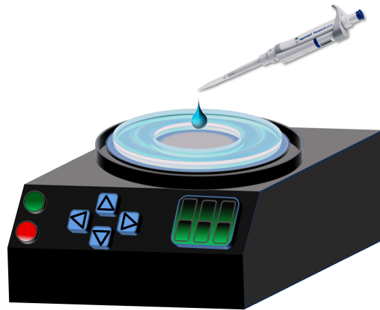
Figure 3.2: Schematic view of a spin-coater which shows that the drop of solution is dispersed on the spinning substrate and forms a film.
