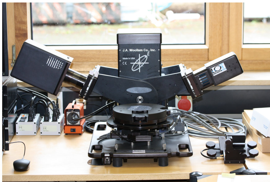
Figure 3.3: Photograph of the Woollam spectroscopic Ellipsometry which was used within the course of the current work for polarization measurements.
