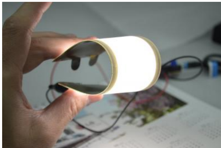
Figure 2.15: A prototype of white flexible OLED lighting panels manufactured by LG chem. [77]
