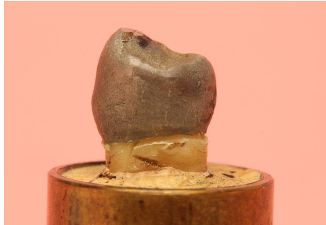
Fig. 20 a: Fracture mode of a specimen with one dentinal wall (buccal wall).
