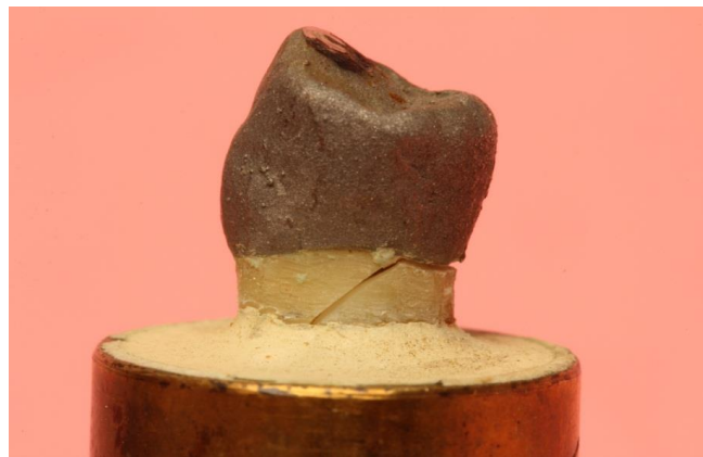
Fig. 20b: Fracture mode of a specimen with two dentinal walls (buccal & lingual wall).
