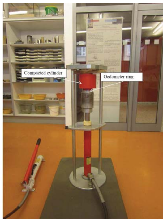
Figure A.2: The sampling of undisturbed specimens (Top) and the sampling of disturbed specimens (bottom)
