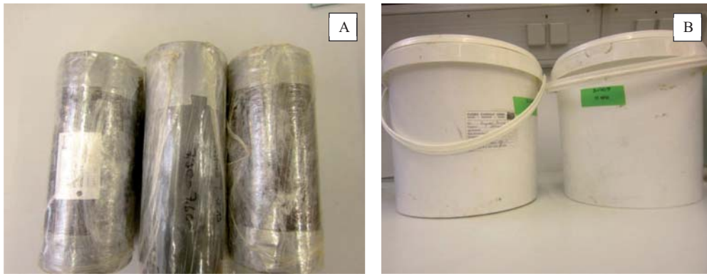
Figure 3.1: [A] Undisturbed samples and [B] disturbed sample packets.
