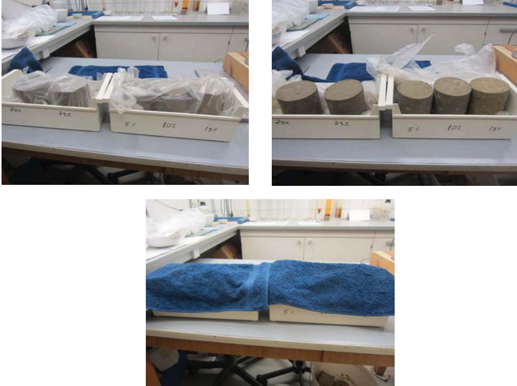
Figure 3.8: The curing of soil samples in ultrasonic measurement.
