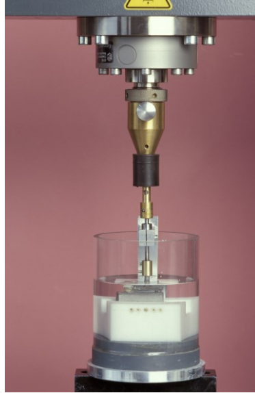
Fig. 10. The specimen (clasp within DRHD) was mounted in the universal testing machine.
