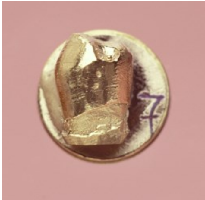
Fig. 12. The replica was attached to an aluminum SEM stub and sputter-coated with gold.
