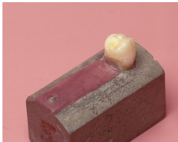
Fig. 4. The unwanted undercut was blocked out, and small piece of wax having hole at its distal end was fixed at the superior surface of the testing model.
