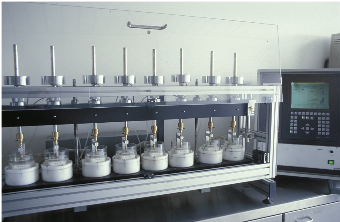
Fig. 11. Clasps within DRHDs were mounted in the chewing simulator device.
