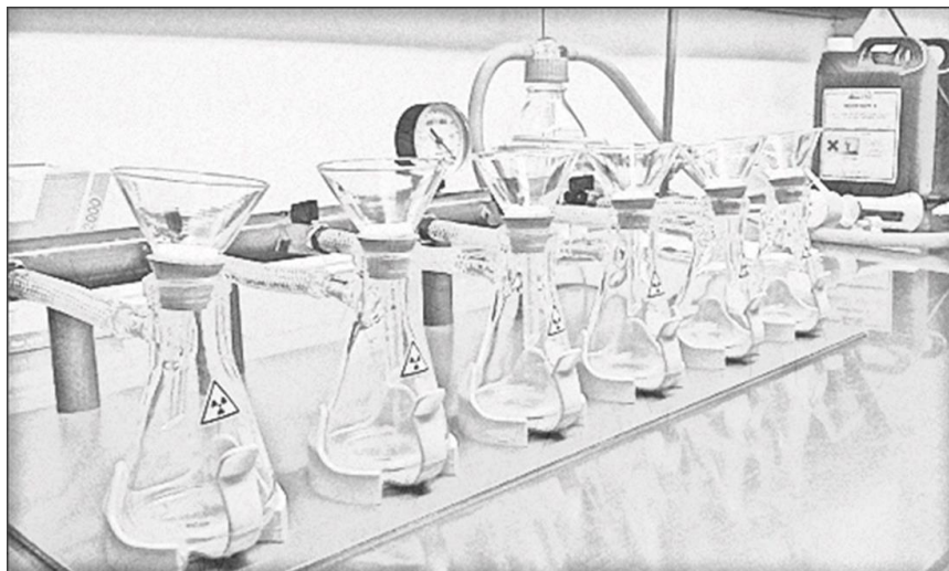
Figure 3.10 | Drawing of the measuring system. 100 ml Erlenmeyer flasks are equipped with Hirsch funnels and connected to an underpressure distribution device. Each flask has its own adjustable valve.
