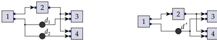
(a) Hyperedge with two dummy nodes (b) Hyperedge with one dummy node
