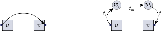
(a) An edge connected to inverted ports (b) Dummy nodes inserted into (u, v)
