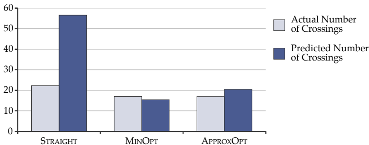
Figure 2.31. Average number of crossings in the resulting drawing when using the given counting algorithm and average number of crossings predicted by that algorithm for the flattened Ptolemy diagrams.
