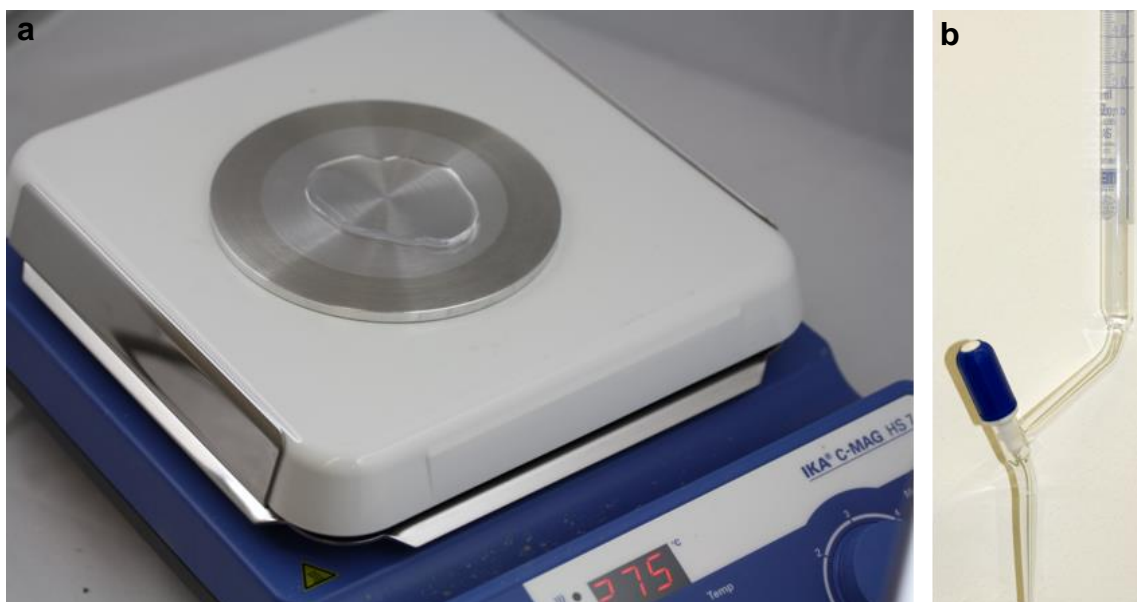
Figure 2.1: (a) hot plate used for nanopowder synthesis by using levitated Leidenfrost puddle on heated aluminum substrate, the solution is introduced to the hotplate by using the (b) 50 mL burette.
