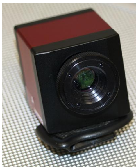
Figure 2.5: Image of IR camera from InfraTec PIR uc 180 with a rate of 24 Hz and a spatial resolution of 40 \mu\text{m}/\text{IR pixel} .
