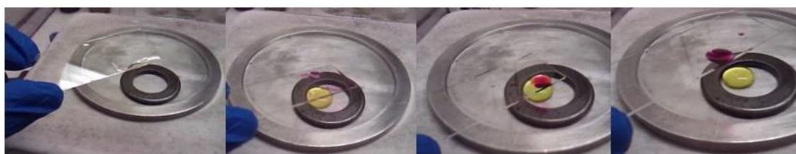
Supplementary Figure S4: Detection of chlorine gas in the vapor: Syringaldazine was placed on a glass substrate and the glass substrate was set above a Leidenfrost drop of \text{AuCl}_4^- solution. A change in the color of syringaldazine from colorless to red-purple indicates a reaction with chlorine in the vapor.
