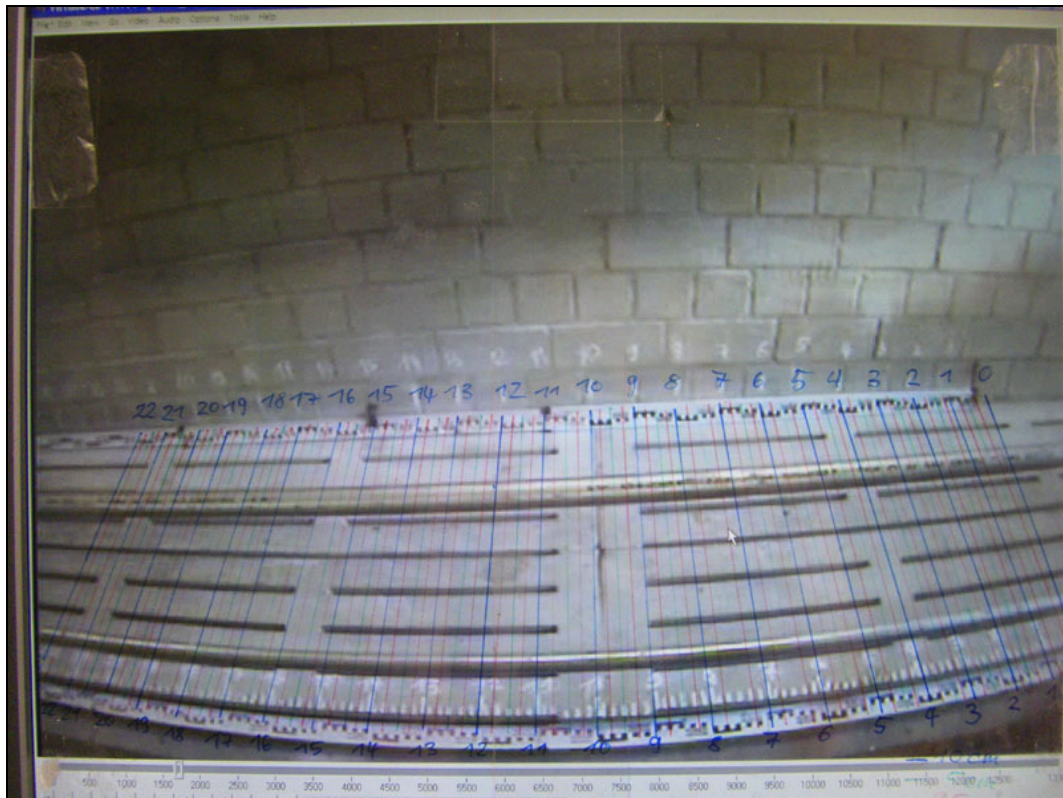
Figure 3: Screen print of the test isle calibrated with yardsticks with the self-made grid (blue, red and green lines) taped on the PC screen for video analysis
