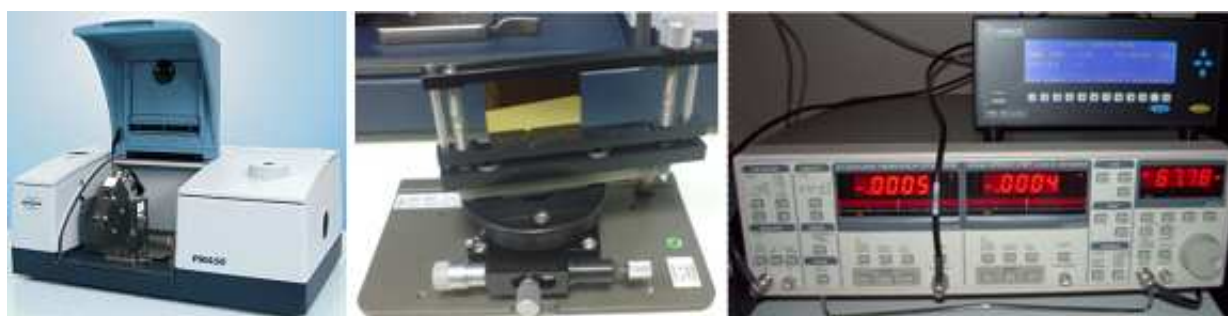
Figure 19: PM-IRRAS instrumental setup. On the left hand side the spectrometer, in the middle the sample holder and on the right hand side the look-in amplifier and PEM.
