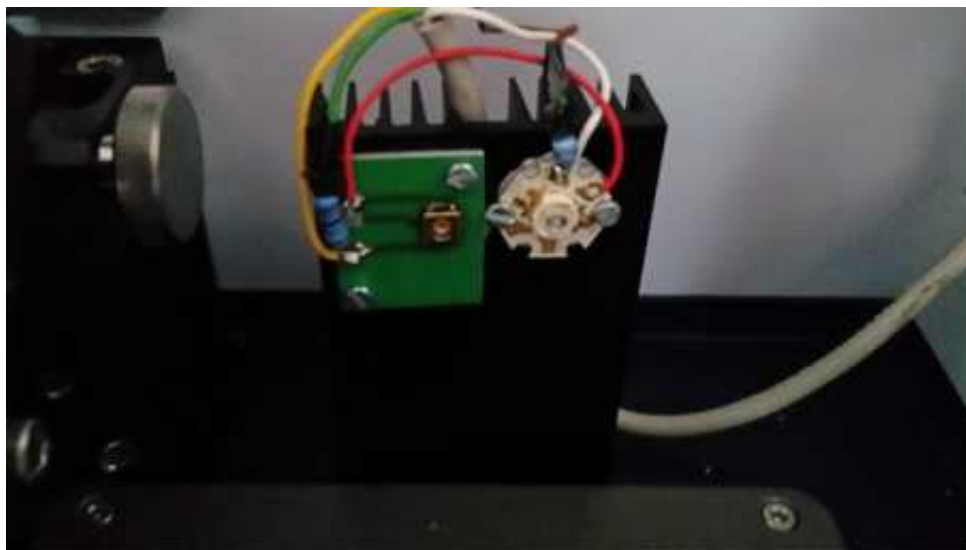
Figure 59: Irradiation-setup in Bruker Vertex 70 PMA-50 spectrometer.
