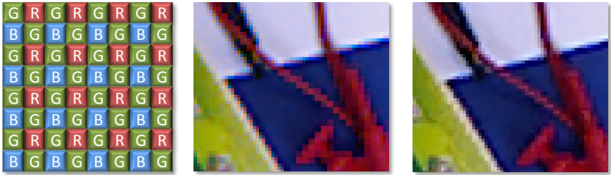
Figure 4.5. Left: an example Bayer pattern (GRBG) as it is used for CCD chips in cameras. Center: the result of the NN demosaicing algorithm shows block artifacts and colored edges. Right: the demosaicing algorithm AHD.
