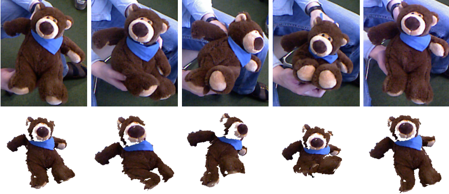
Figure 7.7. Image sequence of a deformed teddy bear. The upper row shows the Kinect color image, the bottom row displays the deformed mesh that was retrieved from the first depth/color image pair of the sequence.
