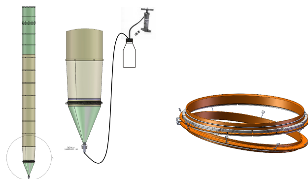
Fig. 4. Left: sketch of sediment trap used in 2011 and 2012 campaigns. The funnel-shaped trap made of TPU foil is connected to the bottom of the enclosure bag via a flange (right panel). Note the tapering of the lowest section of the mesocosm bag. Sampling of sedimented matter is achieved via a silicon tube which connects to a 5 L sampling flask and a hand-operated vacuum pump. Right: flange ring made of laminated fibreglass to attach the external sediment trap to the lower end of the enclosure bag. The upper ring (connected to the bag) is equipped with steel weights to facilitate the sinking of the enclosure bag during mesocosm filling and to keep the bag in vertical position when exposed to currents. Bag and sediment trap are fixed to the upper and lower flanges by stainless steel clamps pressing the TPU foil in notches. Upper and lower flanges are connected with eight screws and sealed with a silicon rubber fitting.
