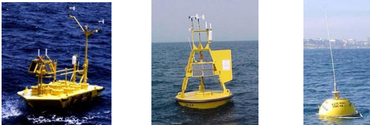
Figure 5.1: Ocean waves (sea surface elevation) measurements devices commonly known as buoys: 6 meter NOMAD aluminium hulled boat shaped buoy (left). 3-meter aluminium hulled discus buoy (center). Data well Directional Waverider buoy (left).
