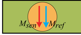
Figure 4.4: The magnetocrystalline anisotropy K_u , M_{sen} and M_{ref} are set perpendicular to the length of the cantilevers during the field annealing for measuring magnetostriction of the sense layer (see section 6.6).
