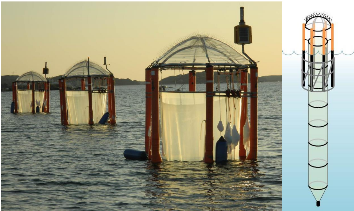
KOSMOS outdoor mesocosms in the Gullmar Fjord, Sweden, and schematic drawing including the underwater part (Photo: J. Bellworthy).
